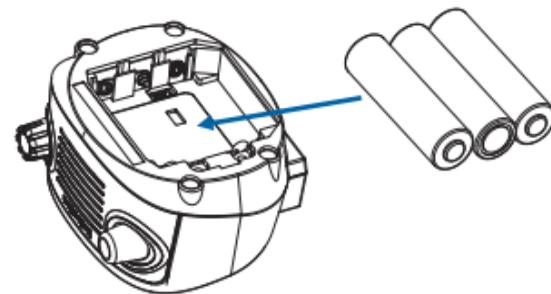
Step3: Reinstall the battery cover and screws. After the batteries are inserted, the GREEN Power LED will automatically light and flash.
