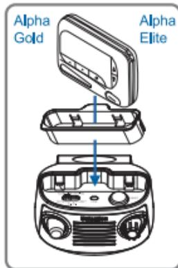
! Before inserting the right pager type dock adapter, please be sure to remove the screws which are fitted inside the socket. After inserting the correct dock adapter, please remember Using the provided screws to secure it.
